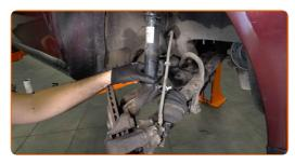
Replacement: strut mount – VW New Beetle Hatchback (9C1, 1C1). AUTODOC recommends:
