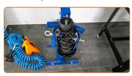
Replacement: strut mount – VW New Beetle Hatchback (9C1, 1C1). AUTODOC experts recommend:
