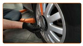
Unscrew the hub lock nut. Use 1-3/16" drive 12-point socket.
