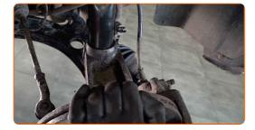
Replacement: strut mount – VW New Beetle Hatchback (9C1, 1C1). Tip from AUTODOC:
