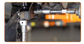
Tighten the lower fastener of the shock absorber. Use a combination spanner #21. Use a drive socket #21. Use a torque wrench. Tighten it to 40 Nm torque.+90°
