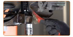
Unscrew the lower fastener of the shock absorber. Use a combination spanner #21. Use a drive socket #21. Use a tap wrench.
