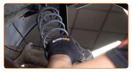
Remove the rubber spring spacer.
