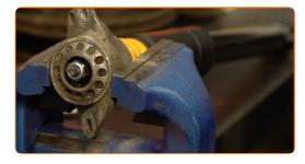
Install the protective cap of the shock absorber mount.
