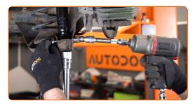
Tighten the top shock absorber fastening. Use a combination spanner #16. Use a drive socket #16. Use a torque wrench. Tighten it to 30 Nm torque.+90°
