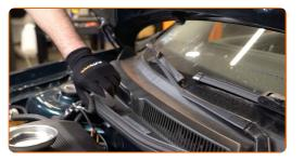
Remove the fender protection cover.
