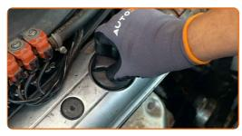
Tighten the oil filler cap.
