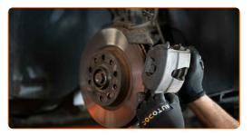
Replacement: brake caliper – VW New Beetle Hatchback (9C1, 1C1). AUTODOC recommends:
