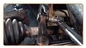
Replacement: anti roll bar links – VW New Beetle Hatchback (9C1, 1C1).
