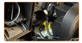
Insert a new filter element into the filter housing. Make sure that the filter edge fits tight to the housing.
