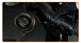
Fasten the clamp on the air intake hose. Use water pump pliers.
