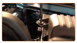
Detach the air intake hose clamp. Use water pump pliers.
