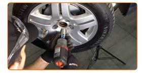
Lower the car and working in a cross order, tighten the wheel bolts. Use a torque wrench. Tighten it to 120 nm torque.
