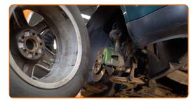
Clean the fastener connecting the tie rod end to the steering knuckle. Use a wire brush. Use WD-40 spray.
