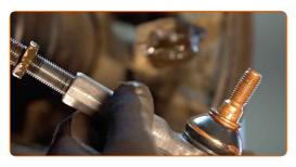
Replacement: track rod end – VW New Beetle Convertible (1Y7). Tip from AUTODOC experts:
