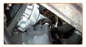
Replacement: engine thermostat – VW New Beetle Convertible (1Y7). Tip:
