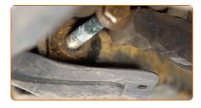
Disconnect the spherical joint from the arm.
