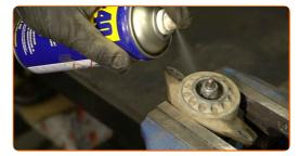
Remove the shock absorber piston rod fastening. Use a drive socket #16. Use a shock absorber socket DDNº6. Use a ratchet wrench.
