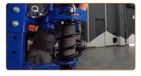
Remove the assembled shock strut.
