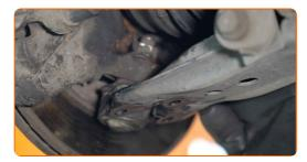
Screw in the fasteners of the ball joint lock plate (3 pieces). Important! Be sure to use new fasteners. Use a drive socket #13. Use a torque wrench. Tighten it to 20 Nm torque.+90°
