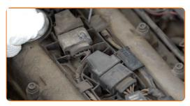
Pry up the ignition coil. Use a crowbar. Use a flat screwdriver.
