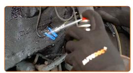
Replacement: brake hose – VW New Beetle Convertible (1Y7). Tip from AUTODOC:
