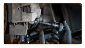
16 Remove the brake caliper.
