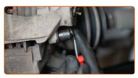
Connect the ABS sensor electric socket. Connect the brake pad wear sensor plug.
