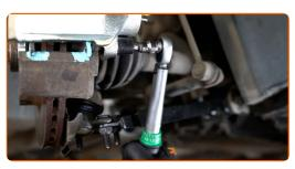
Clean dirt from the brake hose bolt. Use a brake cleaner.
