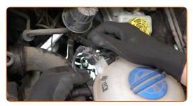
Unscrew the fasteners of the coolant reservoir. Use a Phillips screwdriver.
