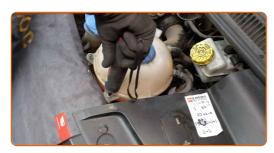
Attach the coolant expansion tank connector.
