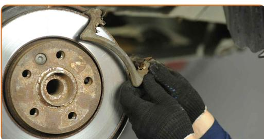
**17** Clean the brake disc fastener. Use a wire brush. Use WD-40 spray.
