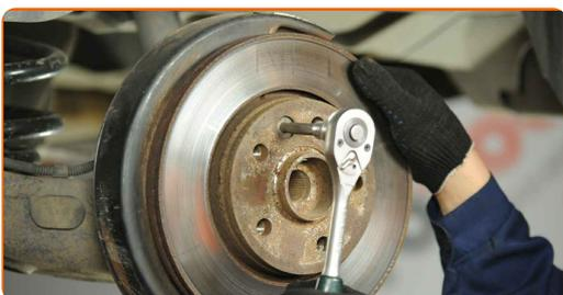
**19** Remove the brake disc.
