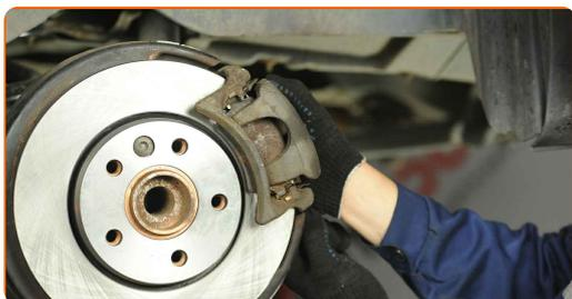
**36.2** Use a drive socket #12. Use a torque wrench. Tighten it to 30 nm torque.
