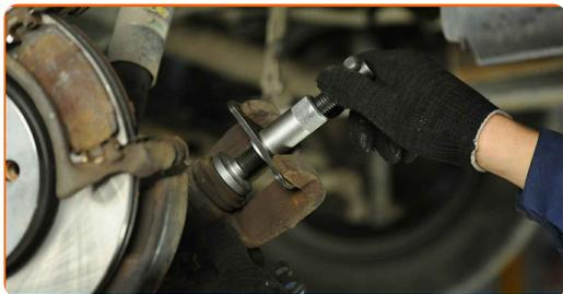
**36.1** Install the brake caliper and fix it.
