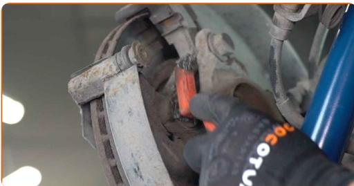
**14** Unscrew the brake caliper bracket fasteners. Use a drive socket #21. Use a ratchet wrench. Use a tap wrench.
