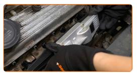
Tighten the ignition coil bolts. Use a drive socket #10. Use a torque wrench. Tighten it to 8 Nm torque.
