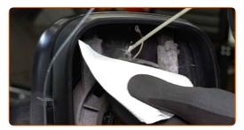
Attach the mirror heating connectors.
