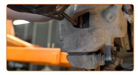
10 Remove the brake caliper.
