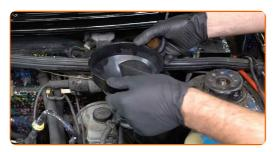
Pour coolant in the coolant reservoir.
