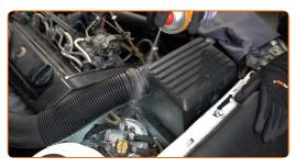
Loosen the fuel filter mounting. Use a drive socket #13. Use a ratchet wrench.
