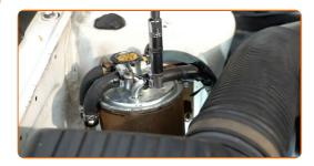
Disconnect the fuel supply lines from the fuel filter. Use round-nose pliers.
