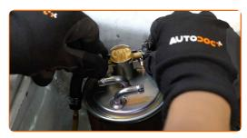
13 Install the fuel line retaining clip.
