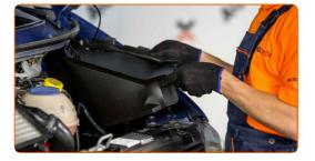
Remove the fender protection cover.
