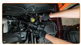
Unplug the mass air flow sensor connector. Loosen the clamp and remove the intake air hose from the filter housing. Use combination pliers.
