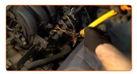
6 Unscrew the intake manifold fasteners. Use HEX No.H6. Use a drive socket #13. Use a ratchet wrench.
