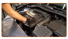
Replacement: spark plugs – VW LT 28-46 II Platform / Chassis (2DC, 2DF, 2DG, 2DL, 2DM). Tip from AUTODOC experts:
