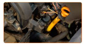
Screw in the oil dipstick bracket. Use XZN #8. Use a ratchet wrench.
