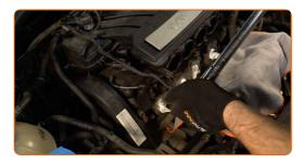
Replacement: spark plugs – VW LT 28-46 II Platform / Chassis (2DC, 2DF, 2DG, 2DL, 2DM). Tip from AUTODOC:
