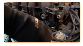
Detach the retainers of the ignition cables.
