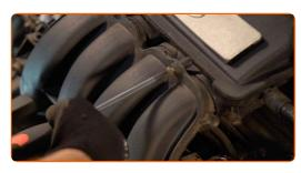
11 Remove the intake manifold.
