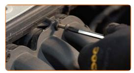
Tighten the intake manifold fasteners. Use HEX No.H6. Use a drive socket #13. Use a ratchet wrench.
