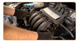
Tighten the intake manifold fasteners. Use a Phillips screwdriver.
