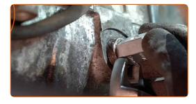
Clean the area around the gearbox housing filler hole. Use all-purpose cleaning spray.
