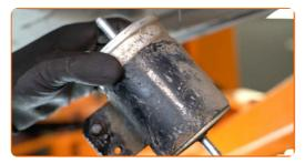
Replacement: fuel filter – VW LT 28-46 II Platform / Chassis (2DC, 2DF, 2DG, 2DL, 2DM). Professionals recommend:
