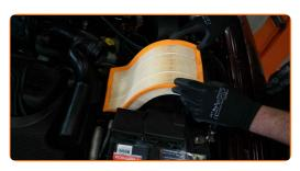
Replacement: air filter – VW LT 28-46 II Platform / Chassis (2DC, 2DF, 2DG, 2DL, 2DM). Tip from AUTODOC experts:
