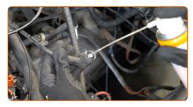
Connect the spark plug wires to the distributor cap.
