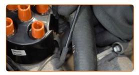
Treat the spark plug wire connectors. Use dielectric grease.
