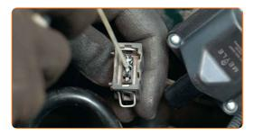
Plug in the ignition coil connector.
