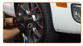
Loosen the wheel hub bolt. Use drive 12-point socket #24. Use a tap wrench.
