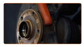
Remove the drive shaft from the wheel hub.
