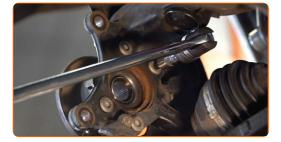
Remove the hub and the bearing together, since they are a sealed unit. Use a crowbar.
