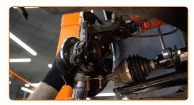
Tighten the hub. Use XZN #12. Use a torque wrench. Tighten it to 70 Nm torque.+90°
