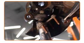
Tighten the ball joint fastening nut. Use a drive socket #15. Use a torque wrench. Tighten it to 60 Nm torque.
