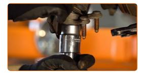
Unscrew the wheel hub axle nut. Use XZN #12. Use a ratchet wrench. Use a tap wrench.
