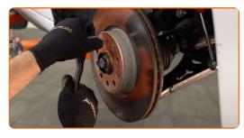
Remove the brake disc.
