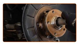
34 Install the brake disc.
