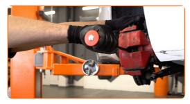
Unscrew the caliper bracket fastening. Use a drive socket #21. Use a ratchet wrench. Use a tap wrench.
