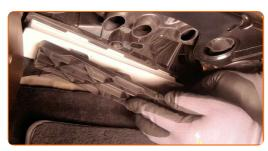
8 Install the bottom cover of the glove box.
