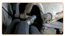
Tighten the oxygen sensor fastener. Use a 22-mm oxygen sensor socket. Use a torque wrench. Tighten it to 37 Nm torque.
