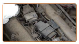
Pry up the ignition coil. Use a crowbar. Use a flat screwdriver.
