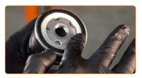
Screw the new filter into its place. Use the 76-14F socket. Use a torque wrench. Tighten it to 18 Nm torque.
