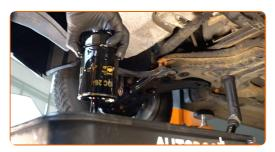
Replacement: engine oil and filter – VW Jetta Mk2 (19E, 1G2, 165). Tip from AUTODOC experts:
