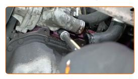
Remove the thermostat housing.
