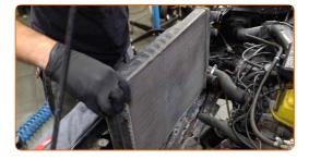
Unscrew the fasteners of the radiator air guides. Use a drive socket #10. Use a ratchet wrench.
