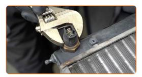
Screw in and tighten the coolant temperature sensor. Use an adjustable wrench. Use a torque wrench. Tighten it to 16 nm torque.
