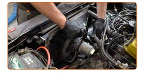
Screw in the fasteners of the fan housing. Use a drive socket #10. Use a ratchet wrench.
