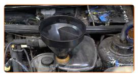
Pour coolant in the coolant reservoir.
