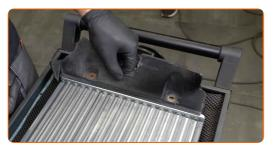
Screw in the fasteners of the radiator air guides. Use a drive socket #10. Use a ratchet wrench.
