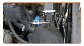
Tighten the radiator fasteners. Use a drive socket #10. Use a torque wrench. Tighten it to 14 nm torque.
