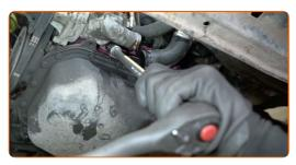
Remove the thermostat housing.
