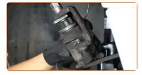
Install the brake caliper and fix it. Use HEX No.H7. Use a torque wrench. Tighten it to 25 Nm torque.
