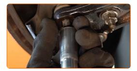
Remove the fastening bolt. Use a drive socket #18.
