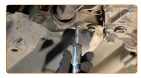
Unscrew the fastener connecting the ball joint to the suspension control arm. Use a drive socket #16. Use a tap wrench.
