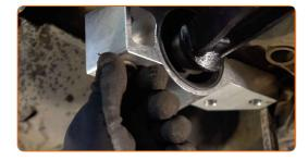
Screw the rear fastener connecting the control arm to the car body. Use a drive socket #18. Use a ratchet wrench.
