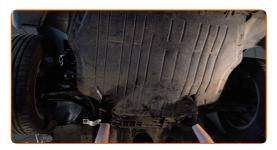
Tighten the fasteners of the oil pan lower cover. Use Torx T25.
