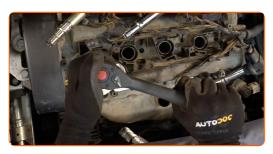
Take out the spark plugs. Use the spark plug socket #16.
