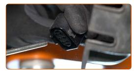
Attach the oxygen sensor connector.
