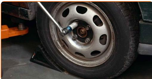
**4** Loosen the fastener of the driveshaft. Use a drive socket #30. Use a tap wrench.
