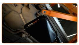
Clean the fasteners of the fuel supply lines. Use a nylon cleaning brush. Use all-purpose cleaning spray.
