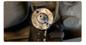
Disconnect the fuel supply lines from the fuel filter.
