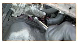
Remove the thermostat housing.
