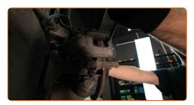
Clean the brake caliper bracket fasteners. Use a wire brush. Treat the brake caliper bracket fasteners. Use WD-40 spray.
