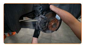
Tighten the brake caliper bracket. Use XZN #14. Use a torque wrench. Tighten it to 90 Nm torque.
