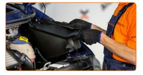
Remove the fender protection cover.
