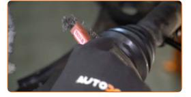
Detach the clamps of the CV joint boot. Use a crowbar.
