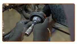
29 Install the CV joint circlip.
