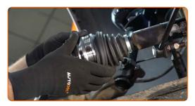
Attach the clamps of the CV joint boot. Use a flat screwdriver. Use clic-R collar pliers. Use a hammer.
